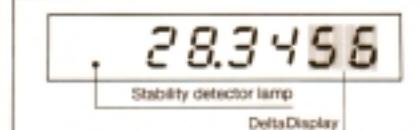
The DeltaDisplay switches on automatically when weighing in substances quickly; the last two digits in the DeltaRange or the last digit in the coarse range is blanked out and the display change sequence speeds up. This allows the increase in weight to be followed better. When weighing in slowly towards the target weight, the two digits (DeltaRange) or the last digit in the coarse range switches back on.
