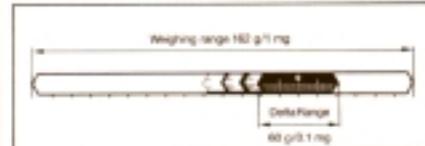
Your AE166 has a coarse range of from 0...162 g; in this range, readability is 1 mg. The DeltaRange (fine range) turns your "milligram balance" into an "analytical balance". This means that the readability is increased to 0.1 mg in a range of 60 g (by pressing tare each time, it can be moved throughout the entire weighing range). Every time the fine range is exceeded, the last decimal goes out; you are then weighing in the coarse range.
